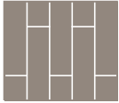
Running laying pattern (at random or regular intervals, depending upon personal choice)
